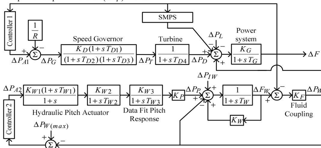
Fig 1. Block diagram of the WEPS model
