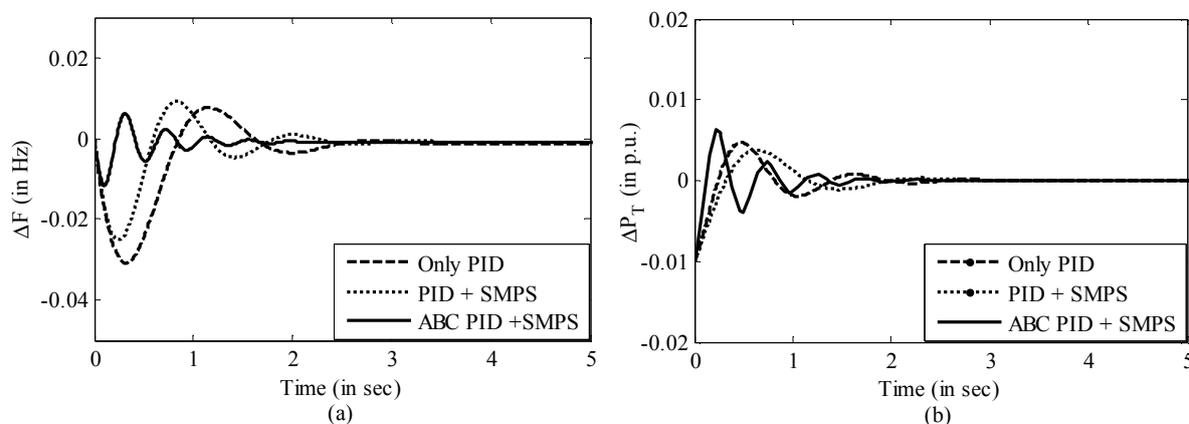
Figure 4. Comparison of different system configuration of (a)  $\Delta F$  (in Hz) and  $\Delta P_T$  (in p.u.) for 1% step increment in load demand and wind speed
