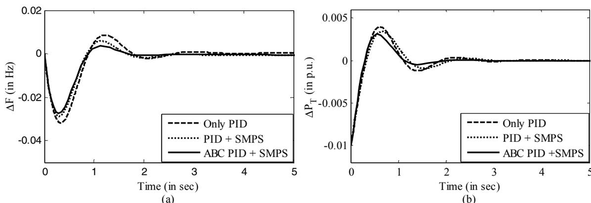
Figure 3. Comparison of different system configuration of (a)  $\Delta F$  (in Hz) and  $\Delta P_T$  (in p.u.) for 1% step increment in load demand
