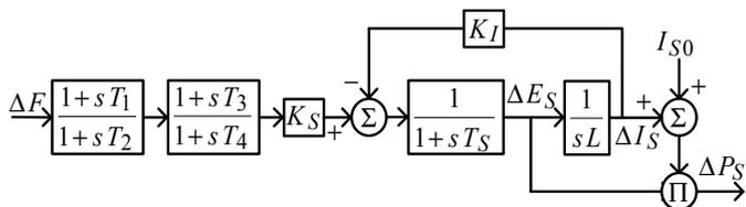
Figure 2. Block diagram of the SMPS model
